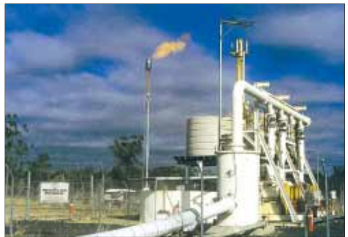
Methane extraction system at Central Colliery coal mine, German Creek. Photo courtesy of NSW Minerals Council
