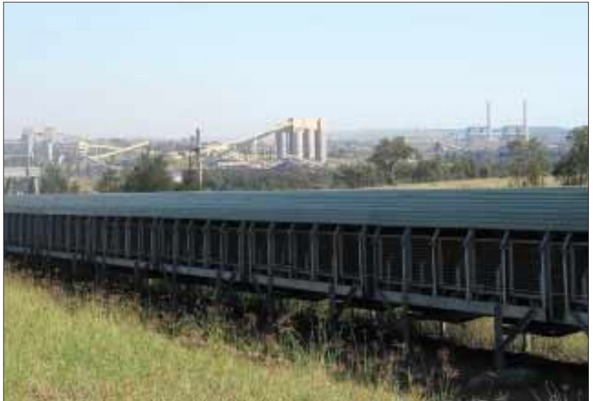
Coal is transported by conveyor directly to the power station. Photo courtesy of Barry Cook
